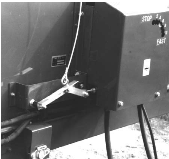
Emergency Stop Tripped
