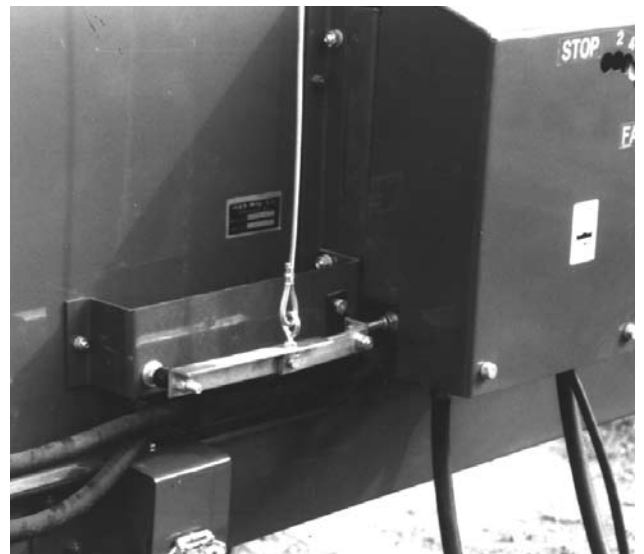
Emergency Stop Re-set
